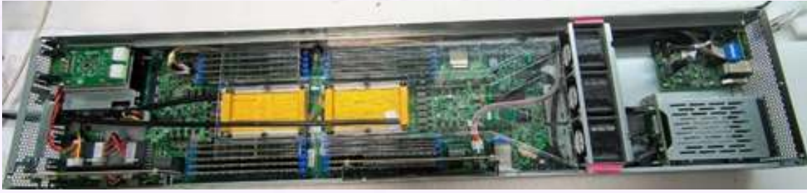
A 330 W coil on chip-based cooling system for Rudra Server
