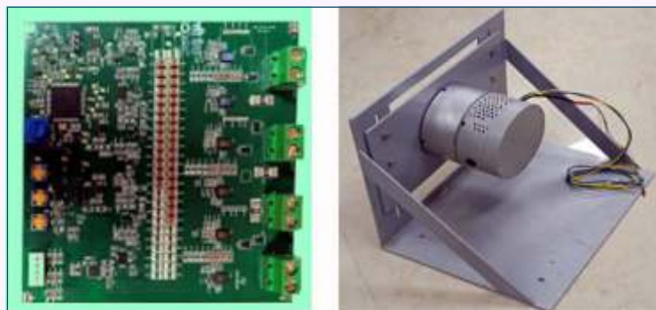
Compact 3 kW GaN based Integrated Drive system for BLDC motor
