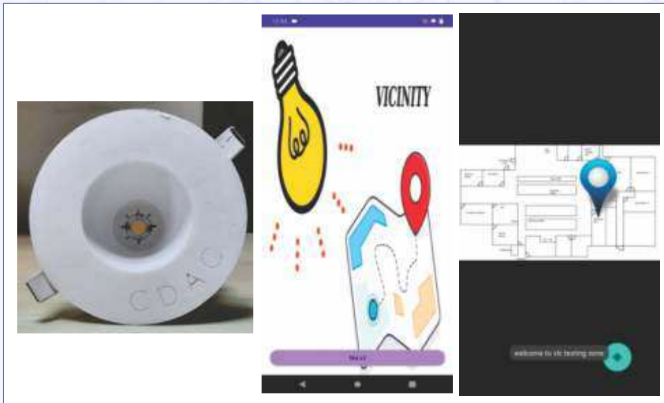
NLoS VICINITY - VLC Transmitter (L) and VLC Receiver ®
