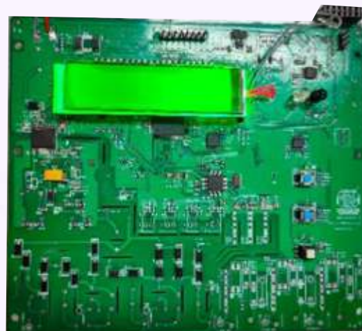
3 Phase Smart Meter PCB using 32-bit COTS MCU
